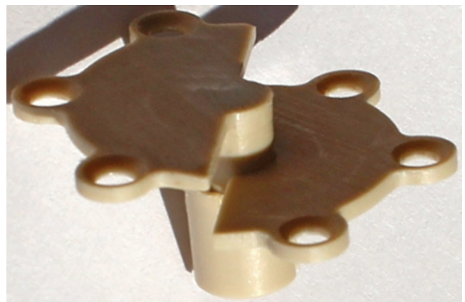
FIG. 3. Side-view photograph of the dynamic telescopic plate with the telescopic portions partially expanded. Figure is available in color online only.
