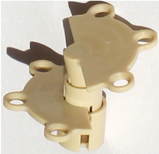
FIG. 4. Side-view photograph of the dynamic telescopic plate with the telescopic portions fully expanded. Figure is available in color online only.
