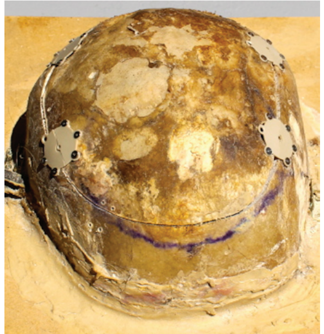
FIG. 7. Photograph of a cadaver skull mounted on a board for testing with the bone flap secured using 4 dynamic telescopic plates. Figure is available in color online only.
